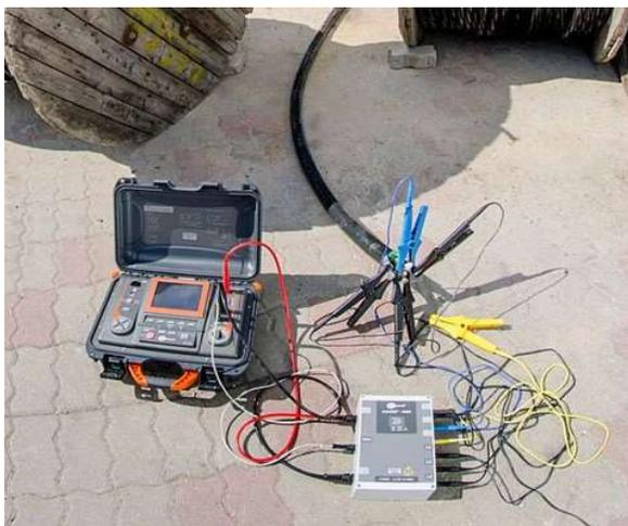
*AutoIso5000 adapter connected to Sonel insulation meter and cable under test*
